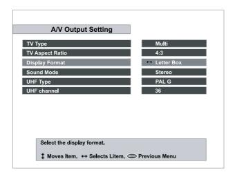
The STB has many A/V Outputs. Control this menu properly according to external components connected to the STB. Configurations concerning Audio and Video can be made here.
